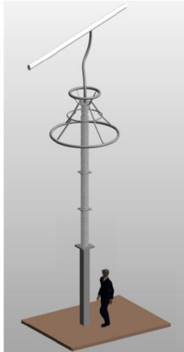
SINGLE SURGE ARRESTOR
